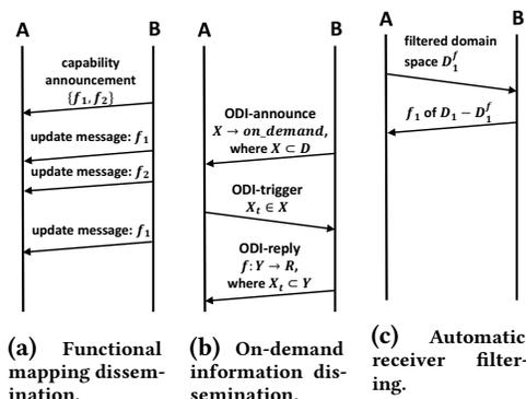
Figure 1: The message-time diagrams of SFP protocol.
